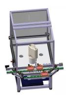
A part of the experimentation facility (The FASTory line) was previously used in a real factory for the assembly of mobile phone components. The FASTory line was retrofitted to simulate its original operations (assembly of Frame, Keyboard and Screen components). It comprises ten workstations, one static buffer cell, and one loading / unloading station. Each workstation includes one main conveyor (main CNV), one bypass conveyor (bypass CNV), and one robot e.g. SCARA robot (SONY SRX-611).
